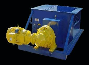
The Rotary Bottle Buster can be designed with many hopper options, including custom feed situations. The Sani-Tech Systems container is used to complete the system. The compacted container will keep product secure from scavengers and can be designed with a drain system to collect any remnants of liquid.
